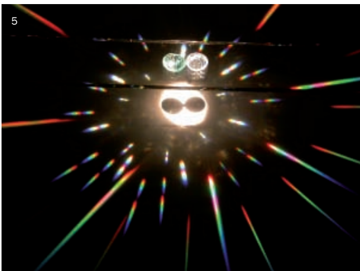
The elongate lithium niobate doubled primaries (b:d 0.7) are instantly separated from the zircon primaries in which the doubled primaries are quite separate at a b:d ratio 1.5. Photograph by Alan Hodgkinson.
