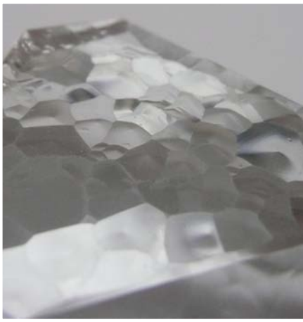
'GROWTH HILLOCKS' ON SYNTHETIC ROCK CRYSTAL ROUGH SURFACE.
