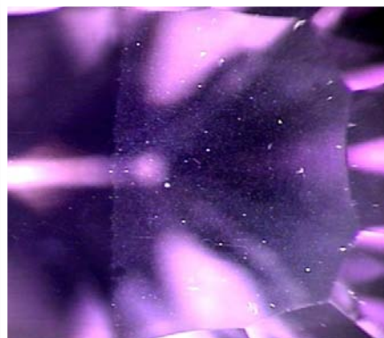
BREAD-CRUMB PLANE IN SYNTHETIC AMETHYST.
