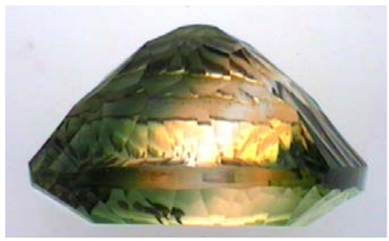
BI-COLOURED SYNTHETIC QUARTZ POLISHED AT 45° FROM THE C-AXIS. THE COLOURLESS SEED CRYSTAL CAN BE EASILY SEEN.
